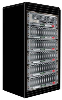
The control of large network servers begins with embedded controllers. Power up, pre-boot services and blade maintenance are performed by low-cost on board embedded controllers.
